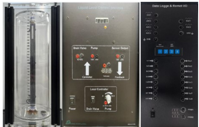
Fig. 2. Liquid-level control system, the interface panel and, data logger.
