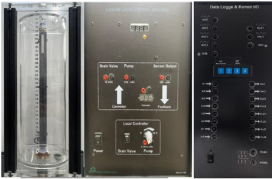
Fig. 1. The system cylindrical tank, interface panel and data logger.
